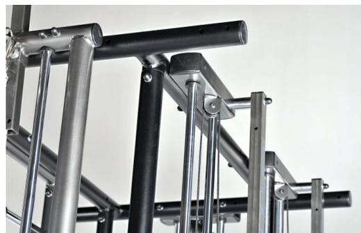
Shown with Cardon Standard Pulley, Speed Pulley, Lateral Pulley and Mounting Ladder
